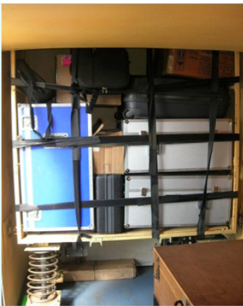
Figure 2: An example of the cases used to protect equipment and the spring shock absorbers used beneath the platforms holding the cases. (Both images courtesy of Krishna Murthy, M.D, Subbakrishna Rao and Prabha Eye Clinic, Bangalore, India.)
